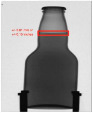
Fill level monitors can measure fill level down to about +/- 0.75 mm (+/- 0.03 inches) for cans containing liquid. Glass containers require a slightly wider aperture and hence have a greater error band (about +/- 3.81 mm or +/- 0.15 inches). Full container x-ray systems have a resolution down to 0.8 mm and that accuracy does not vary by application type.
